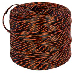
Grip Tight™ Tree Rope is manufactured from a proprietary blend of monofilament polypropylene joined with a spiral wrap. This produces a highly flexible and durable tree rope that will not fray when cut. Our lay-flat design will not damage tree bark, trunk or limbs. Grip Tight™ Tree Rope is more economical when compared to natural fiber rope. Our rope will not mildew, rot and is UV stabilized.
