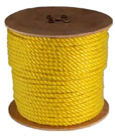
Polypropylene is a lightweight and strong general purpose rope. It is rot proof and unaffected by water, oil, gasoline, and most chemicals. Polypropylene floats yet it is twice as strong as manila. Our regular film polypropylene rope is made with a medium lay, allowing for easy splicing. Harder lay pot warp which is ideal for fishing applications is also available.
