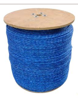
Our heat-treated 12 strand rope with polyurethane coating is torque-free that yields a maximum strength to weight ratio, with the same strength as steel wire rope of similar diameter. This HMPE rope is an excellent replacement for wire rope. Additionally, a specific gravity of 0.98 makes it very useful in a marine environment.
