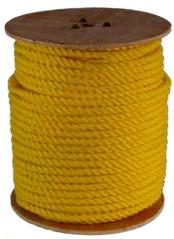
Polypropylene is a lightweight and strong general purpose rope. It is rot proof and unaffected by water, oil, gasoline, and most chemicals. Polypropylene floats yet it is twice as strong as manila. Our regular monofilament polypropylene rope is made with a medium lay, allowing for easy splicing. Harder lay pot warp which is ideal for fishing applications is also available.
