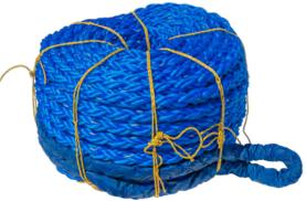
8-strand high strength danline mooring lines, used for mooring larger vessels. These ropes have a high strength to weight ratio, float and do not absorb water. Additionally, they have high resistance to abrasion and chemicals. All our mooring lines are supplied with 6-foot covered eyes on both ends and come with either ABS or Lloyds certificates.
