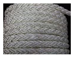
8-Braid plaited nylon plus rope is a non-rotational rope that eliminates hocking and other problems associated with twisted anchor lines. Nylon plus is known for its elasticity and tremendous shock absorbing qualities. Other properties include good abrasion and UV resistance. Additionally, it resists oil, gasoline, and most chemicals. Ideal for use with windlass anchor lines.
