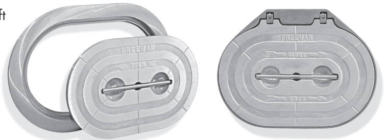
Two 15" X 24" Oval hatches. Left: Lift out style with knife edge seal aluminum ring. Right: Hinged hatch with knife edge seal steel ring.
