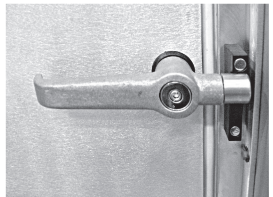
These photos illustrate the knife edge seal and panel mounted gasket (left), and dog/handle detail (right).
